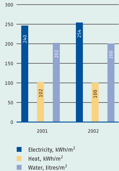
Specific consumption of electricity, heat and water in the real estate owned or leased by Kesko in Finland in 2001-2002
